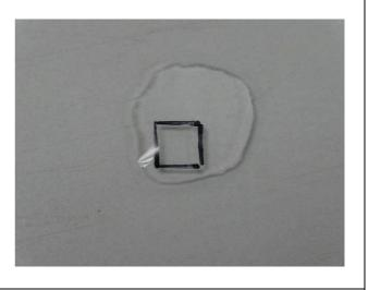
Test Sample (Drop 5~10 cc distilled water )
